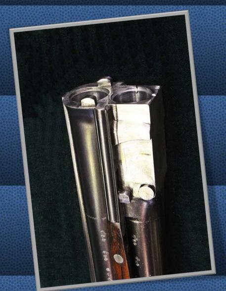
spindle of the top lever that commands the bolt.
