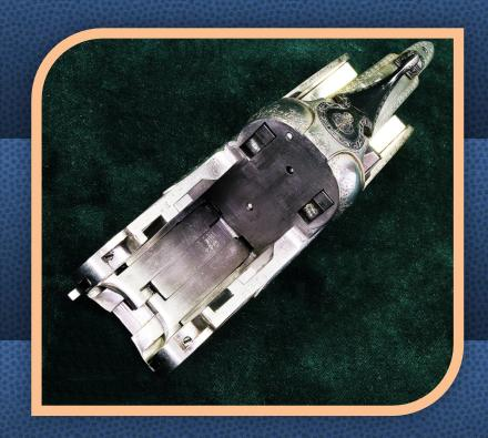
most rational I've ever seen in an old O/U. Two cocking slides on the bottom, two cams that cock the tumblers, the strikers and the
