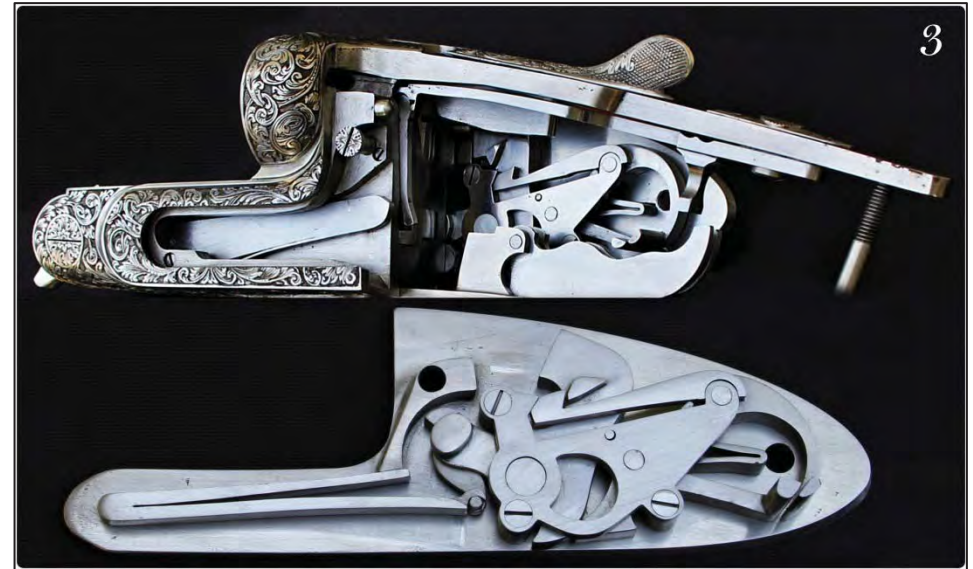
Fig.3)- After the end of the First World War Stefano Zanotti improved the lock, changed the cocking mechanism, added the ejectors and the refined automatic safety.
