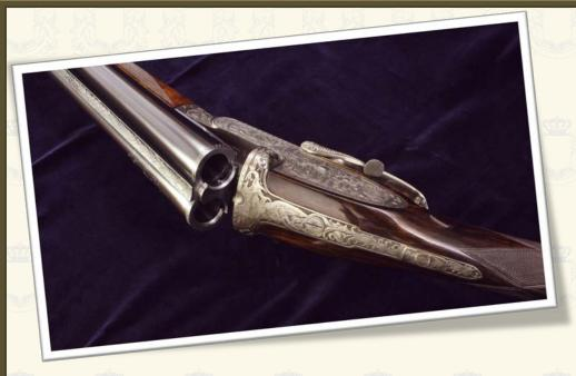
In fact it opens the barrels with that slight friction that only the most tidy adjustment can give, tumblers are gracefully cocked and it closes as a safe. The action proportionate to the gauge and its plans are 2,05" long.
