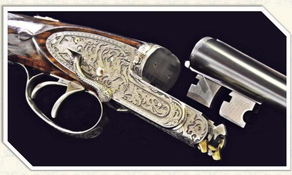
circle, projects from the action when its tumbler is uncocked and retracts whit cocking. Such mechanism avoids every harmful friction among the parts when, wanting to uncock the tumblers, the barrels are closed keeping the triggers pulled.
