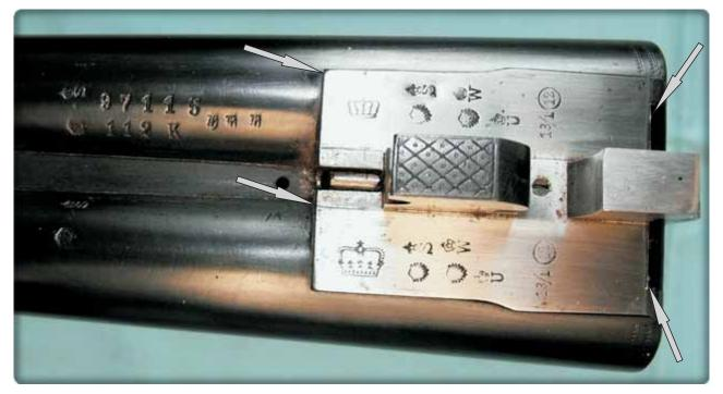
The demibloc system is the most challenging. Barrel, flat and half (longitudinally) of the first and second lump are machined from solid. The two halves are joined.
