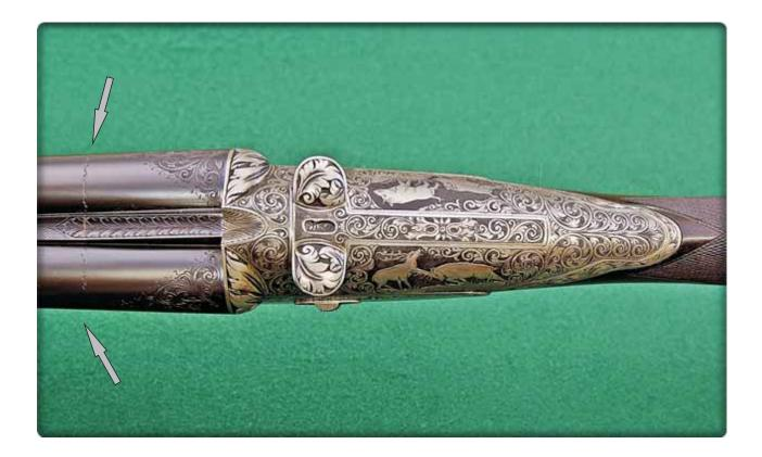
It is possible to find side by side guns that bring higly visible the mark of the union between breech and tubes, at the beginning of the action flats. The tubes, worn, have been substituted while maintaining the original breech, flats and lumps. It is not a <u>monobloc</u> when the lumps are welded to the barrels or together.
