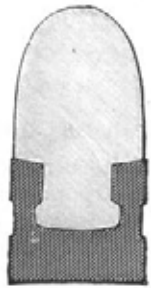
Fig. 1. The New Holland compound bullet for the "Paradox" ball and shot gun, consisting of an aluminium front and a lead base. Reproduced full size.
