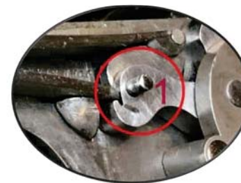
(5). Hammer uncocked. The pin (1) has moved the lever out of the body thus the ejector can operate.
