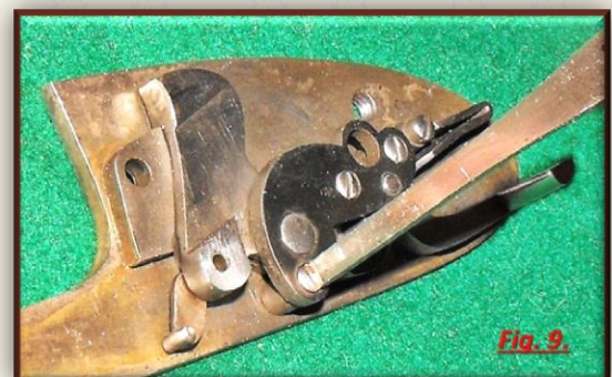
Fig.9. Now it is possible to remove the screws that tighten the bridle. Here they are three, sometimes four and one could be also the sear's pin. The substance is the same.
