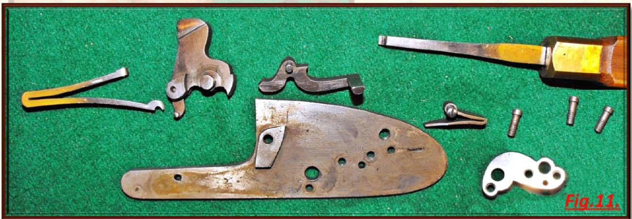
Fig.11. The lock disassembled.
