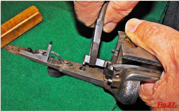
Fig.27. Remove the spring of the lever.
