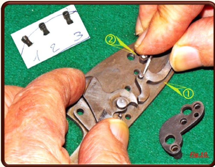
Fig.10. It is important to mind the position of the screws, put them on a piece of paper and sign their position.
