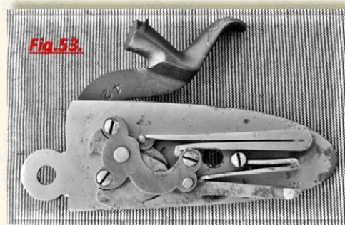
Fig.52. A bar action sidelock. It is fixed to the gun by a notch in the front (1) and by a transit bolt screw.
