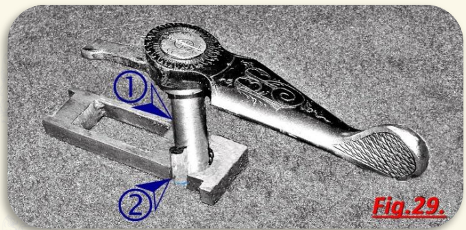
With a long pillar (1) inserted in a slot of the bolt (2). Fig. 28-29.
