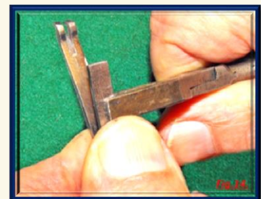
Fig.14. Hold the spring between thumb and forefinger to be able to close it. In this way the clamp finds support on the fingers and doesn't slide along the spring.
