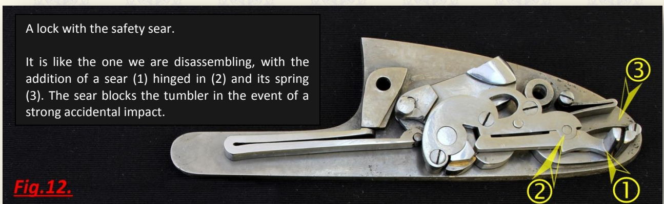
Fig.12. A large-scale lock, known as "Holland & Holland type".
