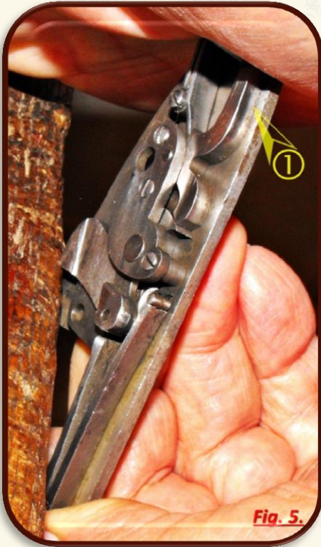
Fig.5. To uncock the tumbler, firmly put its head on the corner of the bench and operate the sear (1). Operate both the sears if they are two, see fig. 12.
