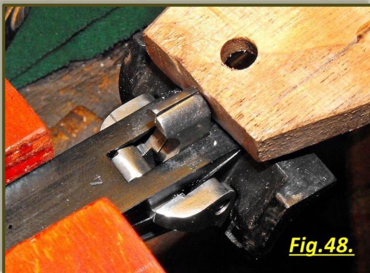
Fig.48. Once reassembled the mechanism, it is necessary to cock the hammers, otherwise the fore-end won't couple with the barrels. To win the springs' force it is better to put the fore-end iron in the vice, lean a piece of wood on the hammers' head and push strongly. It is easier to cock a hammer at a time.
