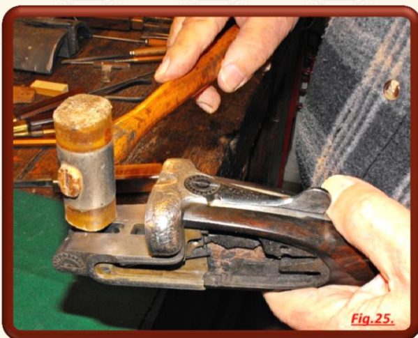
Fig.25. A tap on the action flats and you will feel on the thumb that the action is separated from the stock.
