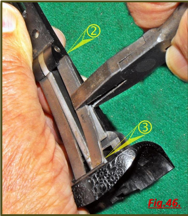
Fig.46. Remove the spring from the joint (2) taking it with the usual clamp. The hammer has to be uncocked.
