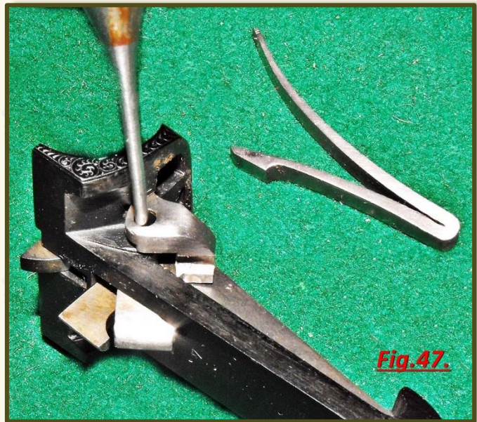
Fig.47. Once removed the springs, remove also the pin of the hammers, now it's possible to extract them from the fore-end iron.
