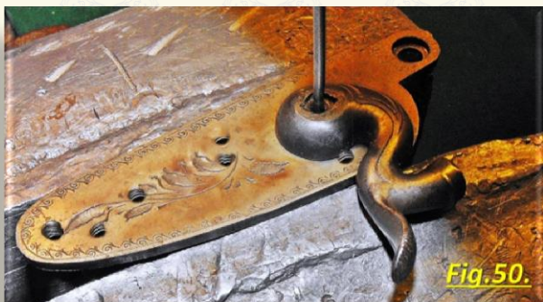
Fig.50. Once removed all the screws and the internal parts, separate the tumbler from the hammer using a drift-punch.
