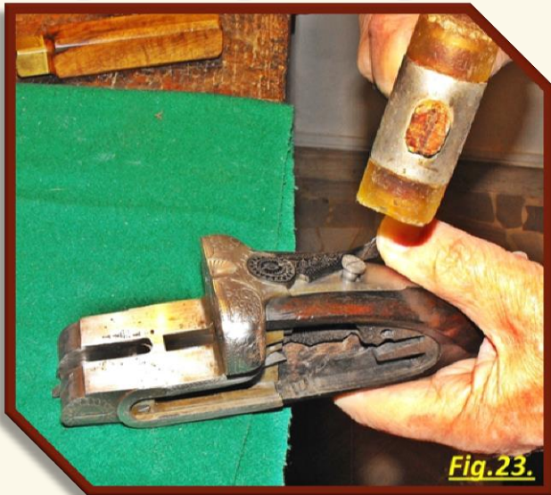
Fig.23. While keeping the lever open, using the thumb (or the piece of wood in the front mortise), put the main screw again in its hole and screw it two turns. A slight tap on the screw's head will remove the triggers plate.
