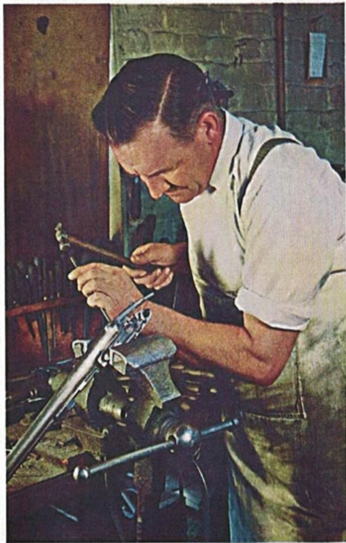
Chasing the Fences on a side-by-side gun.
