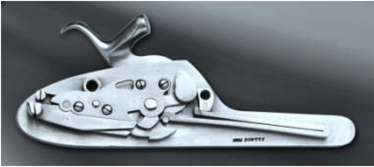
Selfcocking lock with safety-sear. Realized in 1994 by Fabio Piotti.
